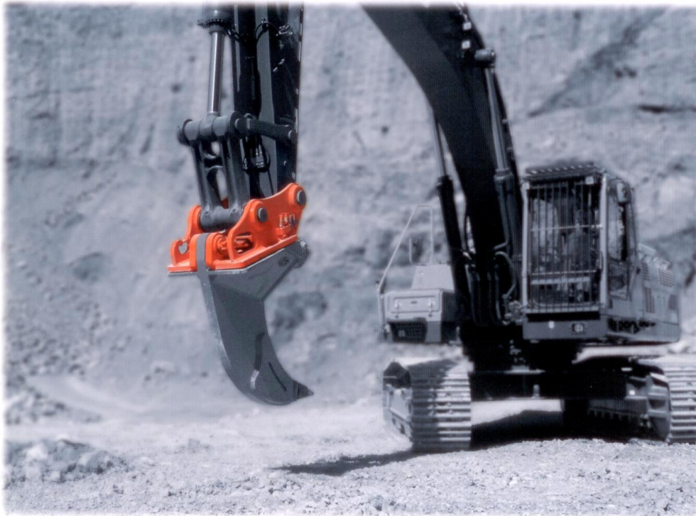
Hydraulic quick coupler with double safety
